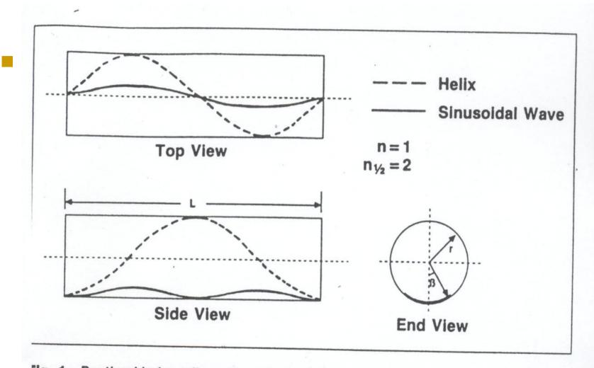
Fig. 1—Postbuckled configuration of pipe in a horizontal hole.
