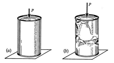
Fig. 9.8 Buckling and crumpling of the cylindrical walls of a can subjected to compressive force.
