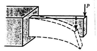
Fig. 9.6 Twist-bend buckling of a deep, narrow beam.
