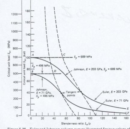
Figure 5.28 Euler and Johnson column curves illustrated for two values of E and  $S_y$  (used in Sample Problems 5.11 and 5.12).
