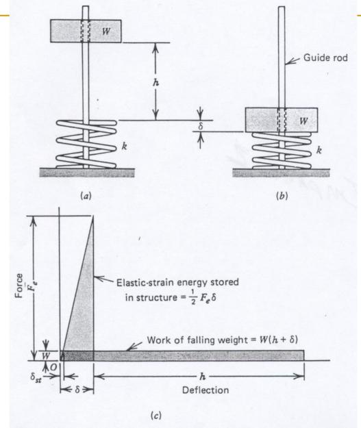
Figure 7.3 Impact load applied to elastic structure by falling weight: (a) initial position; (b) position at instant of maximum deflection; (c) force-deflection-energy relationships.
